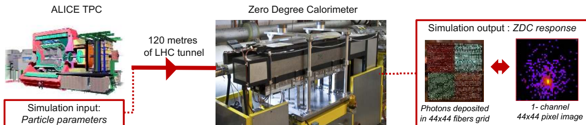
Figure 2.2.1. Fast simulation of the Zero Degree Calorimeter
